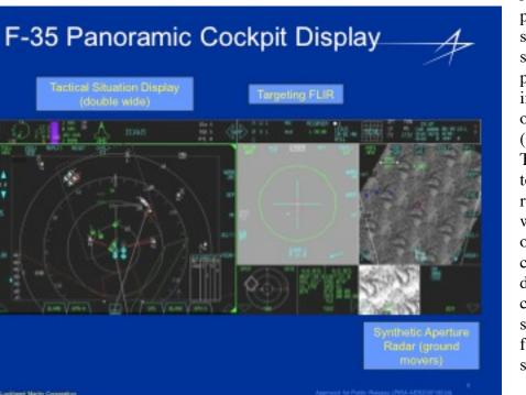
Now, instead of the pilot monitoring a separate display per sensor, fusion presents a single integrated common operational picture (COP) on the TSD. The picture is an easy to interpret graphical representation of what surrounds ownship. It is color coded such that red diamonds, green circles, and yellow squares correspond to foe, friend, and suspect.
