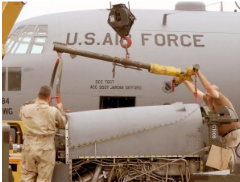
Missouri Air National Guard 774th Expeditionary Airlift Squadron engine mechanics Tech. Sgt. Noel Cardona and Master Sgt. Joseph Ohmes hook up an engine at Karshi-Khanabad Air Base, Uzbekistan, on May 8, 2005, during Operation Enduring Freedom. (U.S. Air Force photo by Tech. Sgt. Scott T. Sturkol
