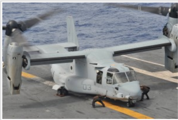
Air department Sailors assigned to the U.S. Navy's forward-deployed aircraft carrier USS George Washington (CVN 73) remove chocks and chains from a U.S. Marine Corps MV-22 Osprey on the flight deck after refueling in support of Operation Damayan. Credit: USN, 11/17/13
