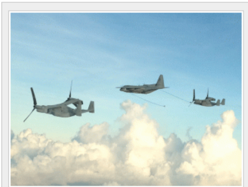
The Ospreys being refueled by a KC-130J. The Marines twin the assets to provide for greater range and endurance in the mission. Credit Photo: Lt. Col Brown
