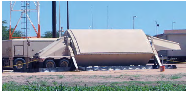
The AN/TPY-2 emplaced and running on generator power. The antenna is in the foreground with the electronics unit behind it.
