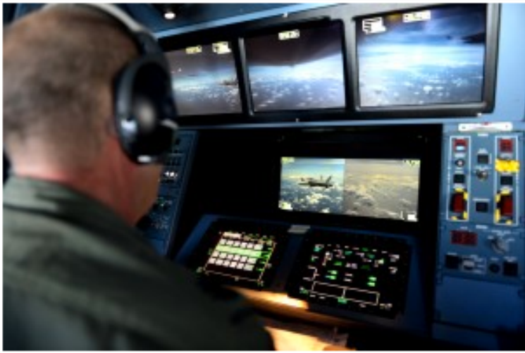
A member of the Royal Australian Air Force refuels a RAAF F/A-18 from a KC-30A Multi Role Tanker Transport while participating in Cope North 13 near Anderson Air Force Base, Guam, Feb. 13, 2013. In the RAAF's new KC-30A, the refuel systems are controlled by an air refueling operator in the cockpit, who can view refueling on 2D and 3D screens. Cope North is an annual air combat tactics, humanitarian assistance and disaster relief exercise designed to increase the readiness and interoperability of the U.S. Air Force, Japan Air Self-Defense Force and Royal Australian Air Force. (U.S. Air Force photo by Senior Airman Matthew Bruch/Released). 2/13/13
