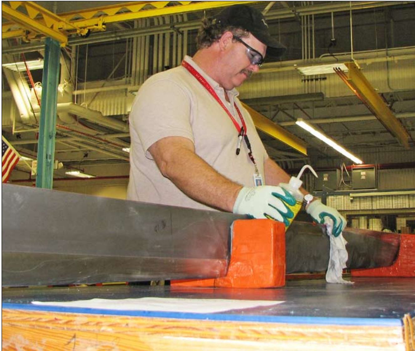
ABOVE: David Greenwood cuts the teeth on a bullgear for the Osprey transmission at the Drive Systems Center. LEFT: Milling Machine Operator Jerry Flores works on a five-axis machine in the DSC’s Large Case Cell, where V-22 transmission cases are machined. BELOW: Mel Caylor, lead bonder in Blade Layup at the RSC, cleans an abrasion strip for a V-22 blade. Photos by Jeff Parish
