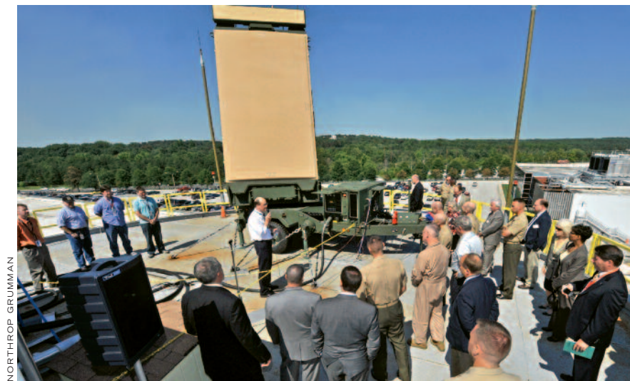
The Ground/Air Task-Oriented Radar (G/ATOR), designed for the Marine Corps as an expeditionary multimission radar, is mounted on a trailer that can be pulled by a 7-ton truck and the Medium Tactical Vehicle Replacement. Northrop Grumman displayed the towable G/ATOR system at its test site at Baltimore-Washington International Thurgood Marshall Airport in September.
