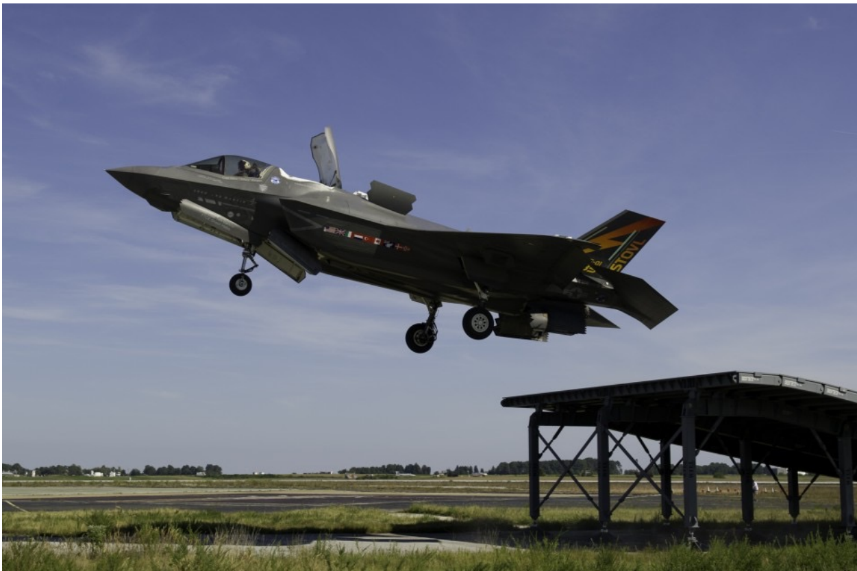
Ski jump testing of F-35B at Pax River. June 2015.
