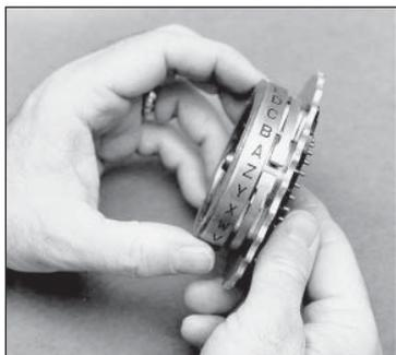
Fig. 1. Setting the notch on ENIGMA
