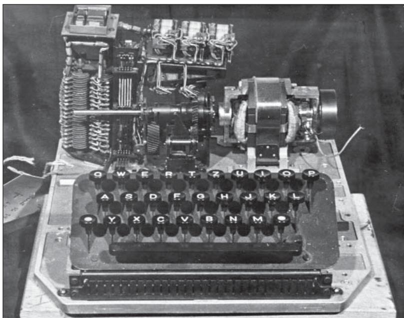
Fig.15. Incomplete Schlüsselgerät 39
