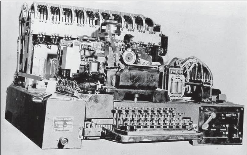
Fig. 13. STURGEON cipher machine
