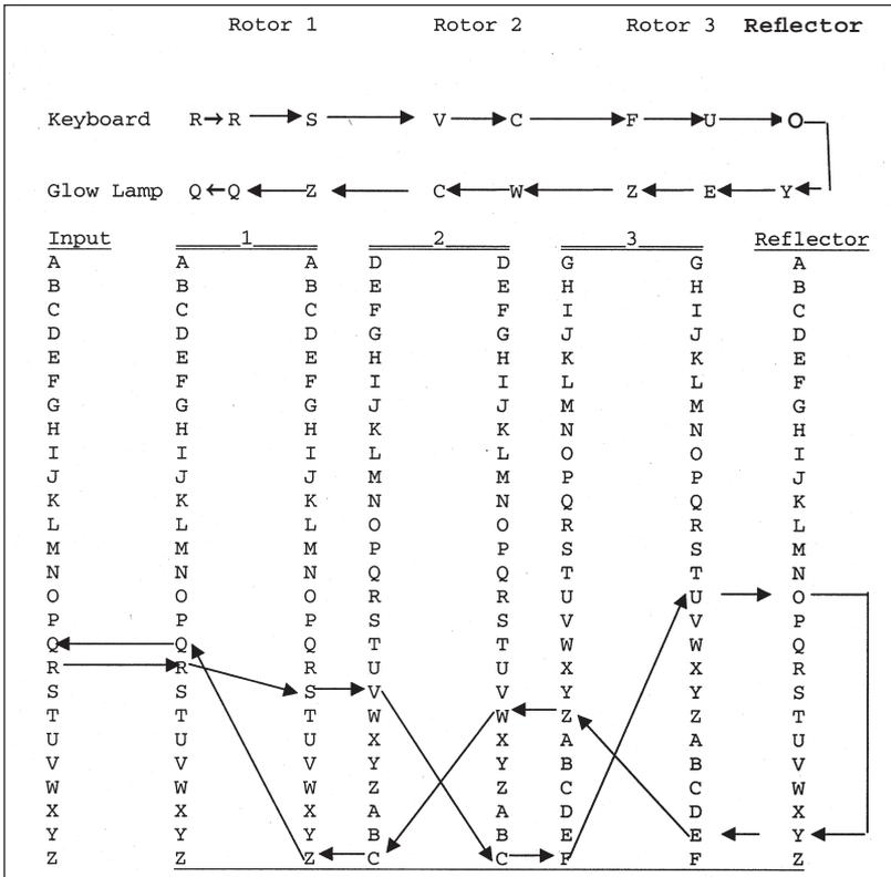
Fig. 6. Sample ENIGMA-type encryption (without stecker). A plaintext R would, in this case, produce the cipher value Q.
