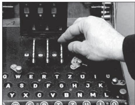
**Fig. 8. Setting the wheels on ENIGMA**
