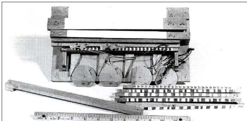
Fig. 23. These models (above and next page) were made by Fritz Menzer to illustrate aspects of the working of the Schlüsselkasten. No actual working devices are available.
