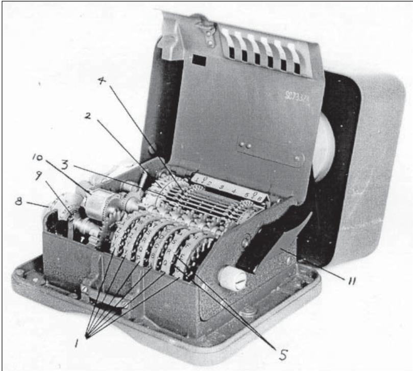
**Fig. 14. The M-209 cipher machine**
