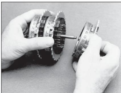
Fig. 2. Assembling the rotor set
