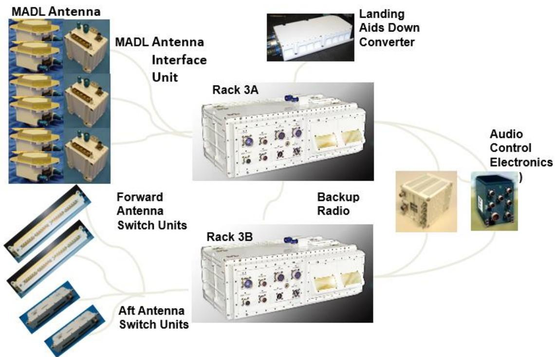
**Fig. 14 CNI system components.**
