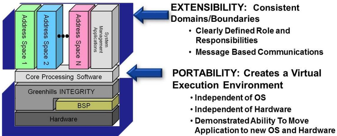
**Fig. 3 Layered software design.**
