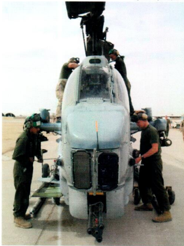
USMC technicians undertake a 200 hour check on an AH-1W operating from Taqqadam operating base in Iraq. Maintenance practices for USMC aircraft are being changed to allow for more “on condition” maintenance, thus increasing operational availability rates.
