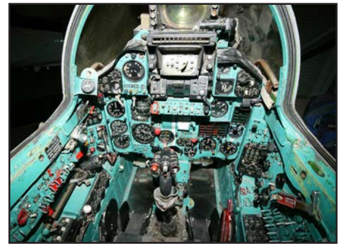
MiG-23 cockpit showing characteristic Soviet-style layout
